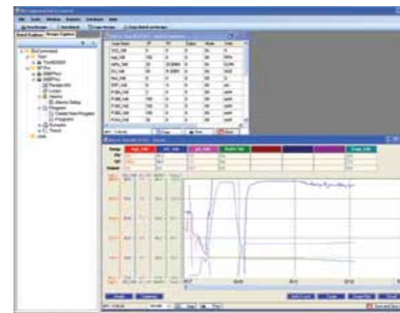
Batch summary screen displays setpoints, current values, and more; custom trend screens allow you to compare and track all of your process data.
