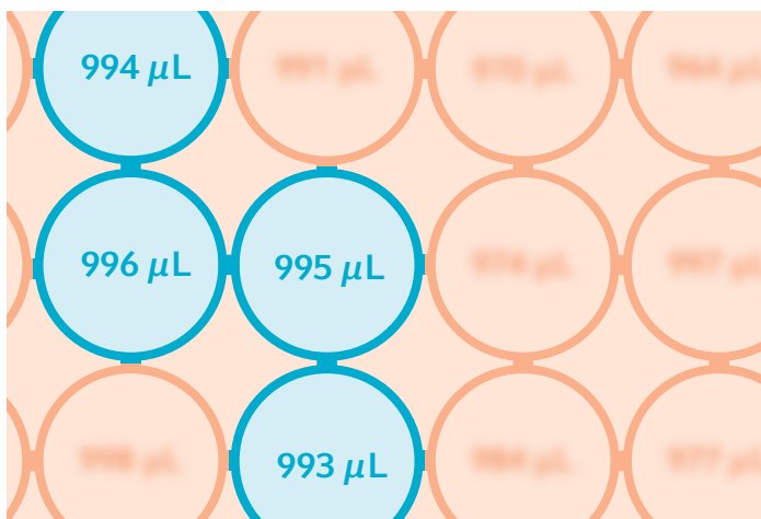
Four measurements – average 994.46 \mu\text{L} , -0.55% systematic error
