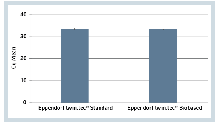
Figure 5: Mean Cq values in qPCR assay with A. baumannii gDNA using Eppendorf biobased and standard twin.tec® PCR Plates (n= 288).
