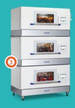
Best conditions for your mammalian suspension cells! The CellXpert CS220 CO<sub>2</sub> incubator shaker ensures precise temperature and CO<sub>2</sub> control, minimized evaporation by active humidity control and reliable shaking. The seamless chamber design and the integrated 180 °C sterilization function protect your cells from contaminations.
