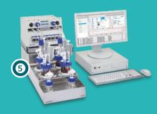
Optimized cell expansion The DASbox® Mini Parallel Bioreactor system provides precise control over culture conditions in a small volume range (100 mL-250 mL), optimizing CAR-T cell growth and viability during the crucial expansion phase.
