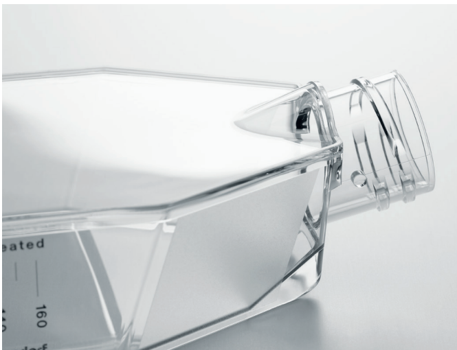
Fig. 1: The ConvexAccess neck of the Eppendorf Cell Culture Flask facilitates access to the growth area, providing protection of the cell monolayer during pipetting. When harvesting cells, increased access also enables better maneuvering with cell scrapers.
