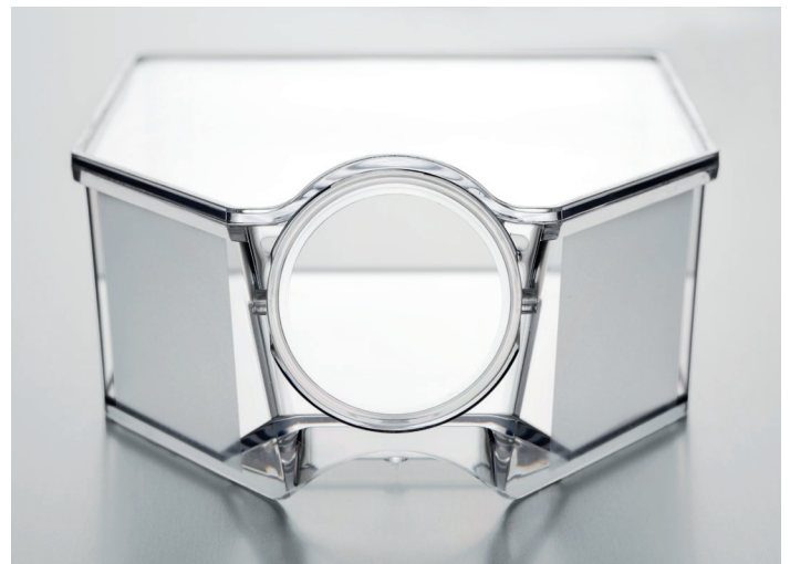
Fig. 1: The ConvexAccess neck of the Eppendorf Cell Culture Flask facilitates access to the growth area, providing protection of the cell monolayer during pipetting. When harvesting cells, increased access also enables better maneuvering with cell scrapers.
