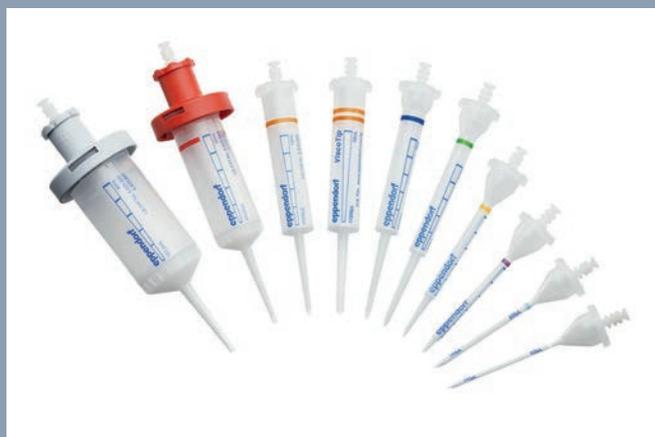
Eppendorf Combitips advanced have been optimized to meet all the needs of any modern laboratory. The Combitips advanced function according to the positive displacement principle, and thus always dispense the correct volume independent of density of the liquid and its flow characteristics (e.g., increased vapor pressure or increased viscosity). Working with radioactive or toxic materials also becomes safer due to the hermetically sealed piston, which prevents aerosol contamination.
