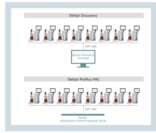
BioFlo 320 with DeltaV Discovery offers a stand-alone solution for R&D laboratories. BioFlo 320 with DeltaV ProPlus PAS allows integration into an existing DeltaV infrastructure.
