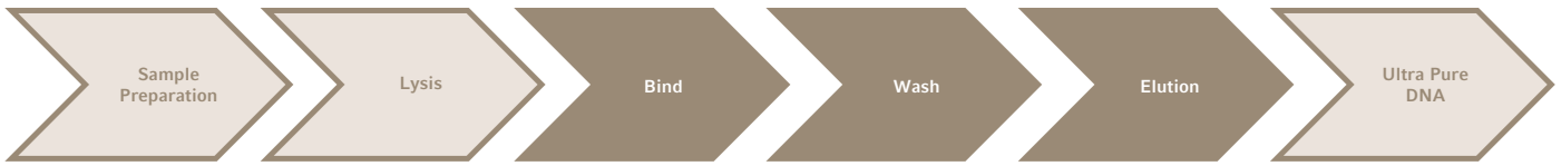
Figure 1: Automated workflow for the Zymo Research Quick-DNA™ Magbead Plus Kit on the epMotion® 5075t. Steps shown in brown can be automated on the epMotion.
