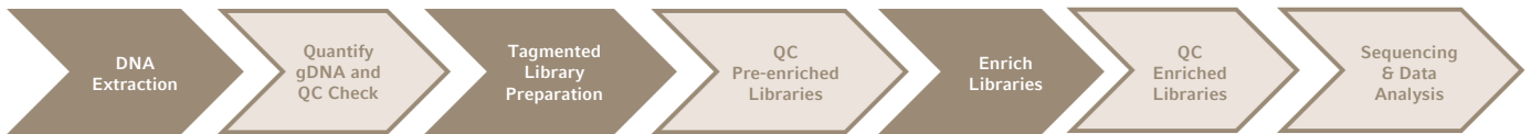
Figure 1: Automated workflow for the Illumina® DNA Prep Kit with Enrichment on the epMotion® 5075t NGS Solution. Steps shown in brown can be automated on the epMotion®.
