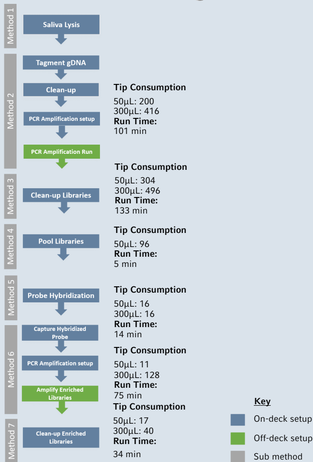
Figure 2: Overview of the sub-methods for the Illumina DNA Prep Kit with Enrichment on the epMotion® 5075t NGS Solution.
