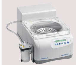
Complete System with an integrated solvent-resistant, maintenance and oil free PTFE pump, and condensation trap. Condensation trap purifies exhaust air by up to 85 %, protecting against unpleasant vapors. At the same time, it extends the service life of all components that come into contact with the vapors.
